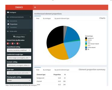
**Above.** Example DMAKS output on average proportions of architectural-element types in all selected analogues. The app allows applying filters to the database on attributes describing the depositional systems and on metadata describing the datasets and the source analogue studies.
