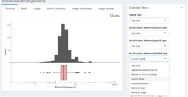
**Below.** Example DMAKS output on the proportion of different types of facies units in the filtered analogues, and for selected types of elements.
